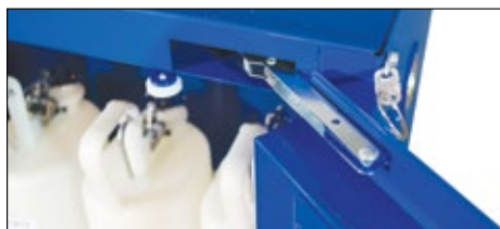
Encased self-closing mechanism provides obstruction-free access to top shelf space. Fusible link melts at 165°F (74°C) to automatically close door(s) under fire conditions.
