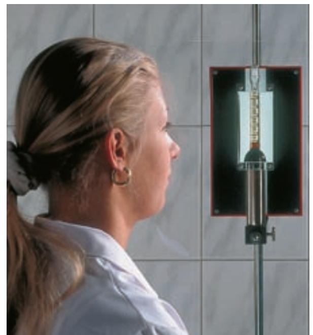
Fig. 6 Measured values can be reliably and accurately read off with the aid of a safety reading lamp
