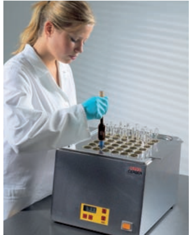
Fig. 5 The butyrometers are brought to the exact reading temperature in a water bath
